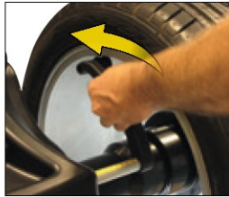
Quick selection and rim run-out measurement with internal data gauge.
